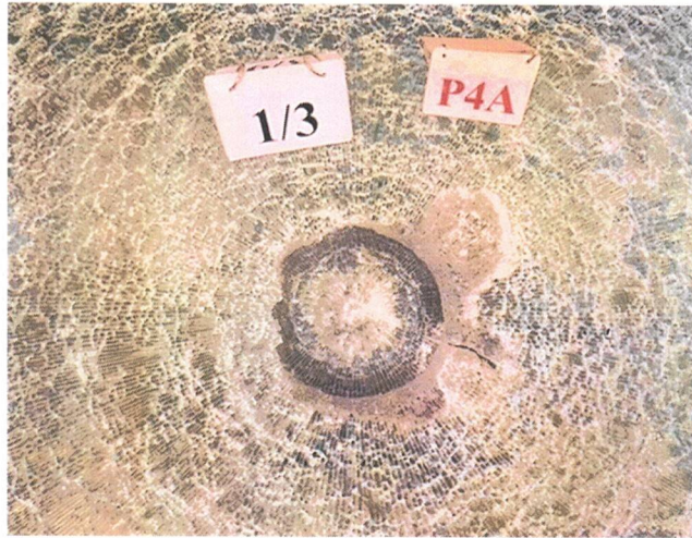
test piece No. 1 after 3 rd impact
